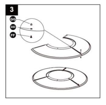
Attach reflector plate (B) to reflector panels (A) using M6 x 8mm screws (FF), Φ6 washers (DD) and cap nuts (GG). Secure loosely with cap nuts (GG).
