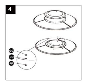
5. Attach reflector assembly to head assembly (C). Secure with cap nuts (GG) and  $\Phi 6$  washers (DD).
